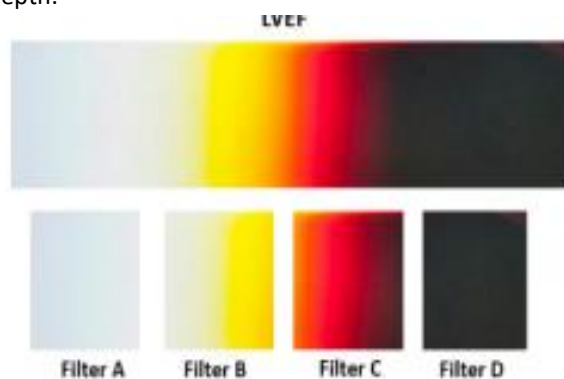
Figure 1. The primary sections of the LVEF are created by a rigorous cutting procedure
